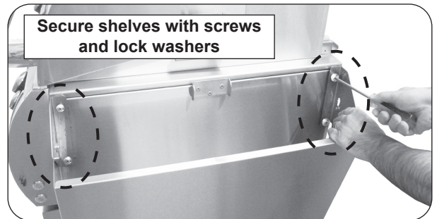
Fig. 13-2 Install folding shelves
