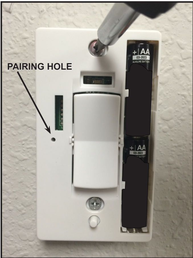
Figure 3. Mounting IFT-RC150 Wireless Wall Switch
