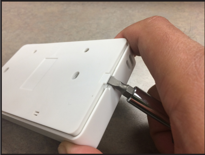
Figure 2. Wall Switch Disassembly
