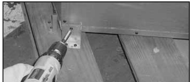
Figure 3.11 Removing Shipping Brackets
