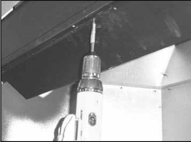
Figure 8.1 Remove Smoke Shield
