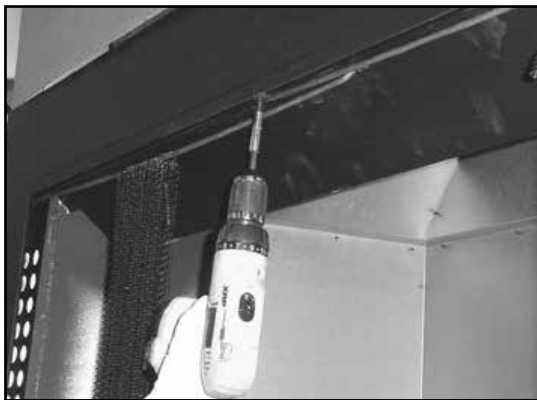
Figure 3.8 Remove Screen Rods
