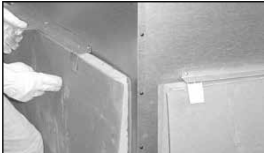
Figure 3.6 Unpack Back Refractory
